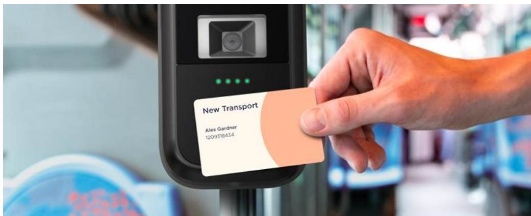
Figure: Passing a smartcard in front of the NFC antenna
