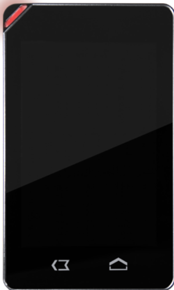
Blinking red Low battery
