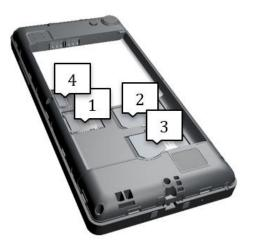
1 SIM1 slot 2 SIM2 slot 3 SAM slot 4 SD card slot
