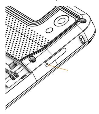
The tray has one slot on the TOP and one slot at the bottom compatible with Nano SIM 4FF.
