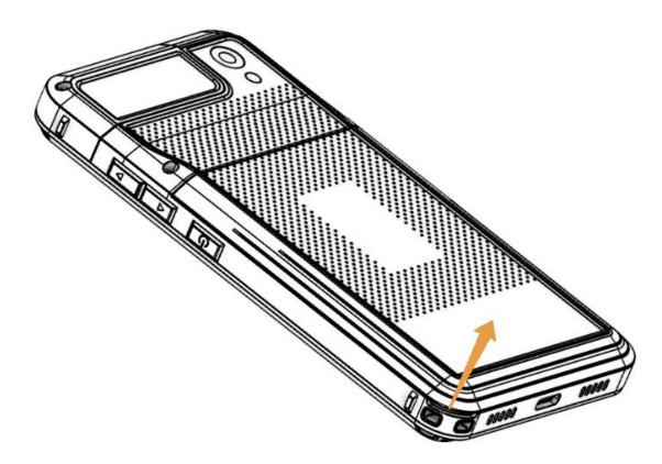
2. Use the small nook on the bottom to remove the battery.
